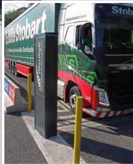
LEFT: RingGo, a cashless parking solution and part of the Parkmobile Group, enables motorists to check parking space availability BELOW: WheelRight Tyre Pressure Technology system, capable of measuring tyre pressures on any vehicle without the need for any mechanical intervention
